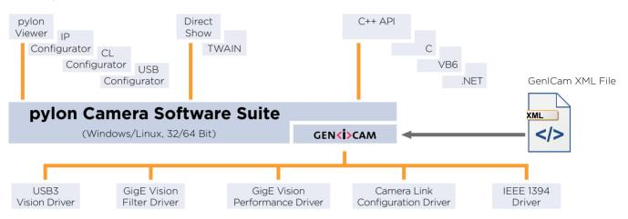
The architecture of the pylon Camera Software Suite is based on GenICam Technology, which offers you easy access to the newest camera models and the latest features. Changes to an existing camera device in your application essentially become a plug-and-play process.
